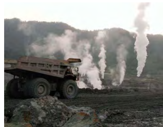
The Ladolam Mine. To extract ore from the fluid-saturated ground of this mine, the ground must be cooled artificially by water injection and steam release. According to Simmons and Brown, the active magmatic-hydrothermal system at the Ladolam mine could have formed the large gold ore deposit over the past tens of thousands of years.
